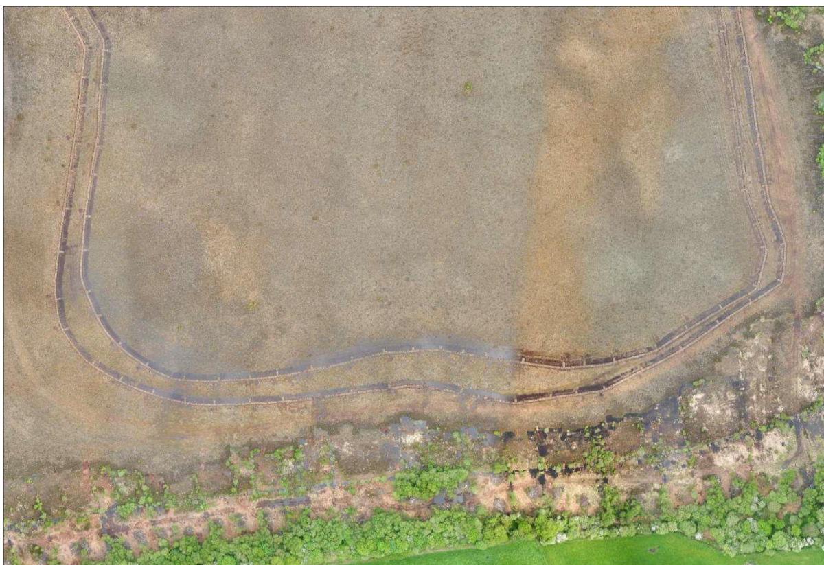
Figure 5.5 Example of high-resolution ortho-imagery illustrating contour bunding on the high bog
