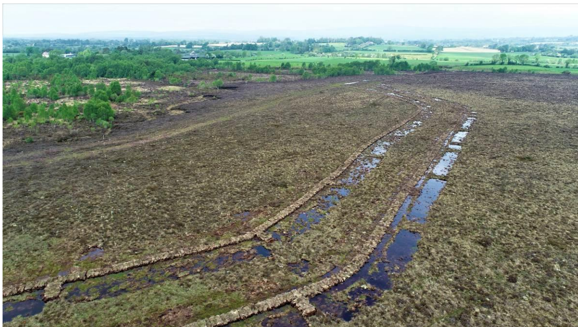
Figure 5.6 Example of contour bunding on the high bog illustrating finger bunds extending perpendicular to the main bund
