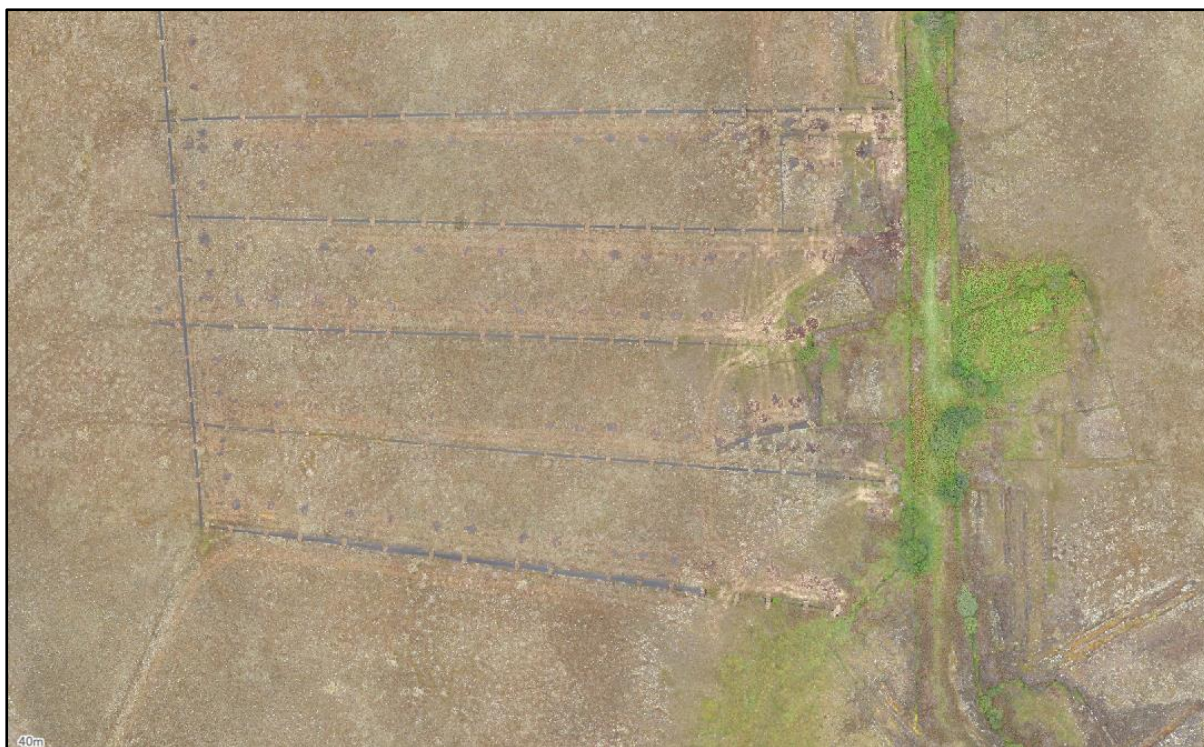
Figure 5.4 Example of high-resolution ortho-imagery illustrating peat dams constructed on the high bog.
