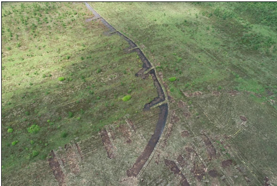
Figure 5.6 Example of oblique imagery illustrating contour bunding on the high bog
