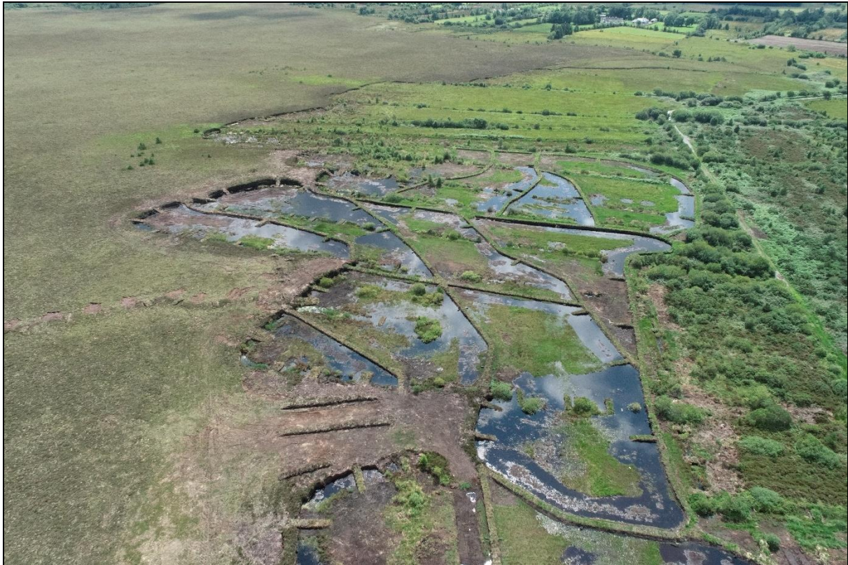
Figure 5.7 Example of oblique imagery illustrating cell bunding on cutover illustrating finger bunds extending perpendicular to the main bund
