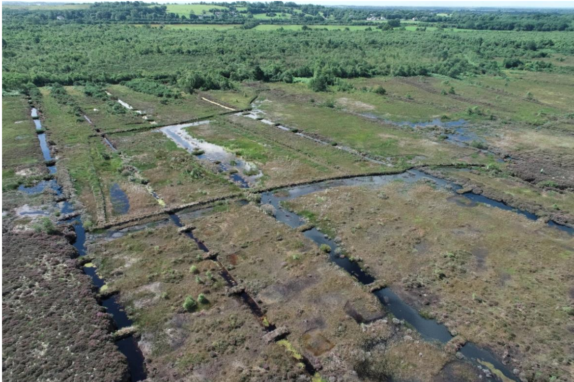
Figure 5.5 Example of high-resolution ortho-imagery illustrating peat dams on the cutover
