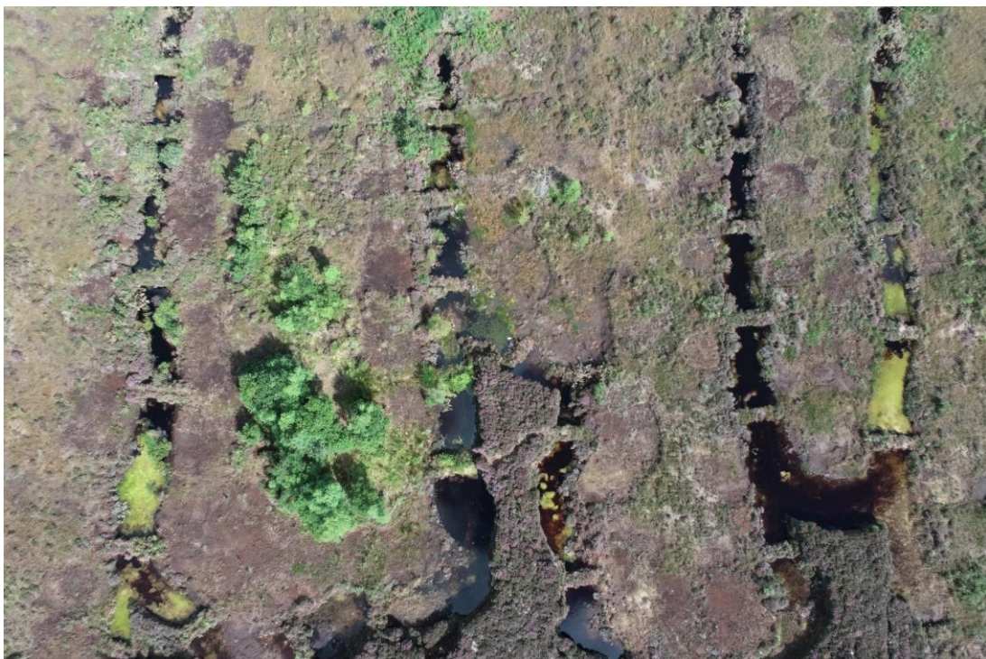
Figure 5.6 Example of cell bunding on the cutover bog illustrating water table close to the ground surface
