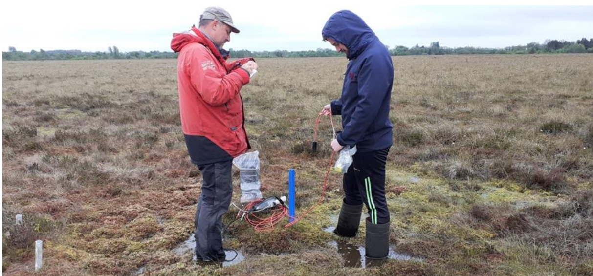
Figure 5.2 Monitoring (dipping) of piezometers in Ballynafagh using electronic dipper, April 2021
